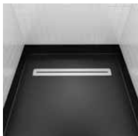
BLÜCHER® WaterLine Vinyl To be placed minimum 5 cm from wall to long side and minimum 10 cm from walls to ends
